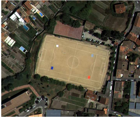
Figure 2.4. ICC Banyoles (Spain) ICC test field with man-made canvases deployed (June 2005).
