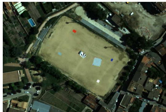
Figure 3.4. ICC Banyoles (Spain) ICC test field with man-made canvases and Siemens stars deployed (July 2008)
