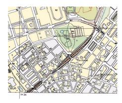
Above image shows the generalization of shared lines in polygon boundaries. The result, where the boundaries are not coincident, is not visible at 1:10.000 scale.
