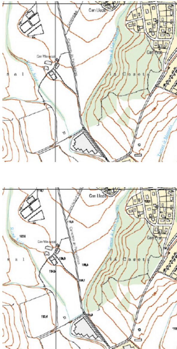
Figure 11.- Top image shows the data generalized automatically at scale 1:10.000. Manual editing is required as is showed in the bottom image.
