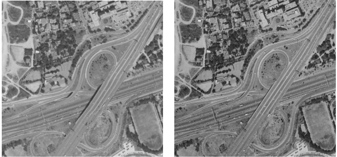
Figure 2.- Left image shows an orthophoto rectified using a DTM, right image shows the same orthophoto rectified using DSM.
