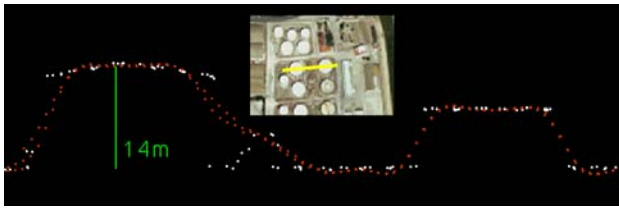
Figure 4: Differences between LIDAR points (white) and DEM grid points (red)
