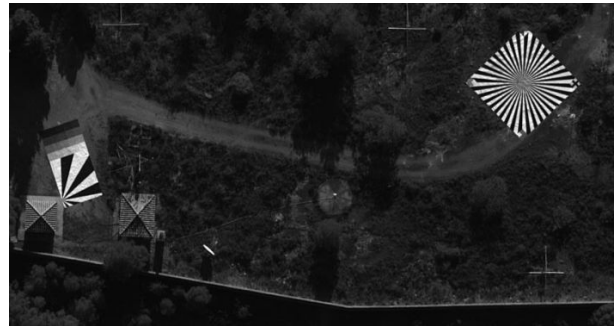
Figure 5: Siemens star target used for the resolution study
