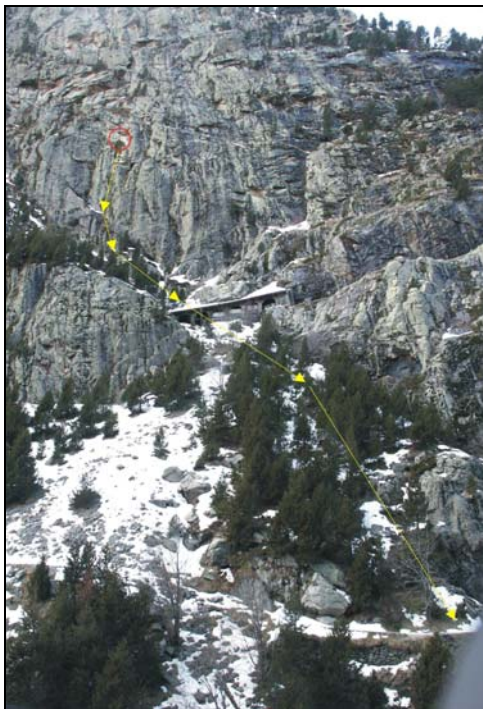
Figure 6: Rock fall occurred in 3rd March 2003. In yellow the path followed by the rock fall.
