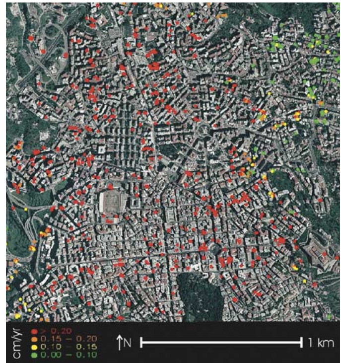
Fig. 4. Full-resolution coherent pixel (circles) map superimposed to an optical image of the Vomero zone (courtesy of CIRAM). The false-color representation within the circles is relative to the estimated deformation mean velocity expressed in centimeters per year.
