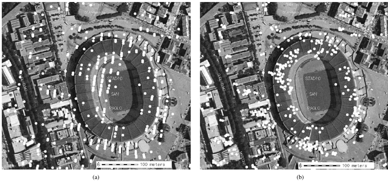
Fig. 8. Location of the coherent pixels relative of the San Paolo Stadium (a) without and (b) with topographic correction shown in (11). An optical image of the stadium is on the background.
