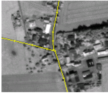
Figure 6. Line extraction of a road intersection. The different road segments are topologically connected by a node.
