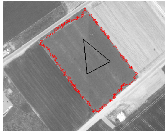
Figure 3. Parcel extraction example with starting polygon (black) and extraction result without smoothing (red)
