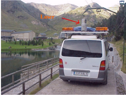
Figure 16: Integration of a terrestrial laser scanner in the GEOVAN
