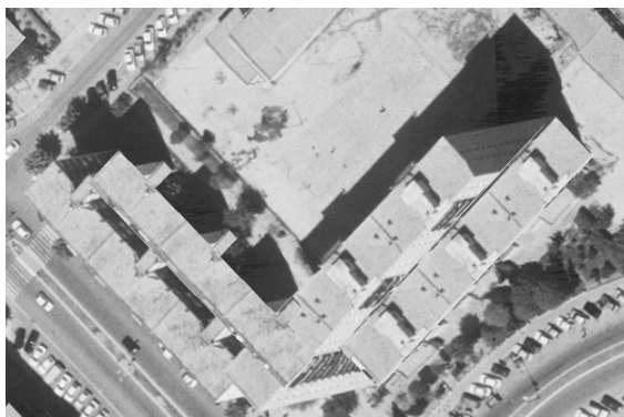
Figure 3. Standard orthorectification without hidden parts removed
