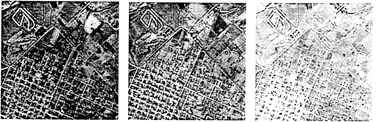
Figure 3. Detail of the fusion by the LHS method in R (left), G (center) and B (right) bands
