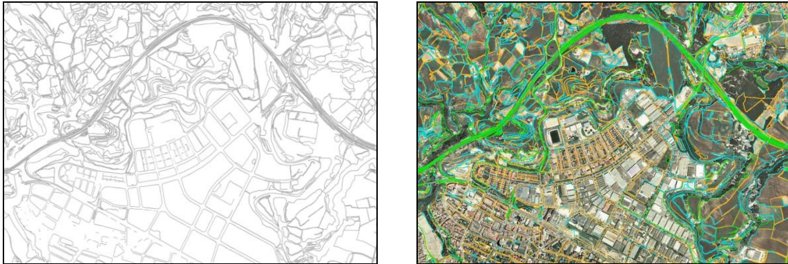
Figure 9. Urban area: on the left, the original break lines; on the right, the classified break lines on top of the image.
