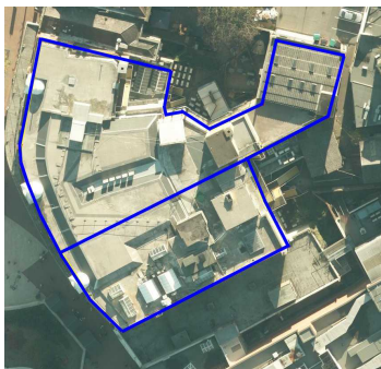
Fig 6. The 3D roof level structures clearly do not match with the 2D footprint
