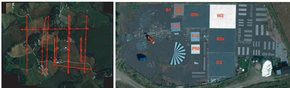
Figure 2. Left: Flight lines in Sjöckulla on 1 September, 2008. Right: Radiometric and spatial resolution targets at Sjöckulla test field. B1: Black gravel; R1: Red gravel; B2a: Black gravel, version a; B2b: Black gravel, version b; G: Grey gravel; W2: White gravel; P20, P30, P50: portable reference reflectance targets with nominal reflectance of 0.20m 0.30 and 0.50.
