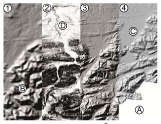
Fig. 2 – shaded relief from ArcGIS:  $\mathcal{O}$  Gtopo30 oblique light  $\mathcal{O}$  SRTM slope  $\mathcal{O}$  SRTM oblique light  $\mathcal{O}$  DGM5 oblique light
