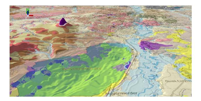
Figure 2 – final geological model of the Berzdorf region.
