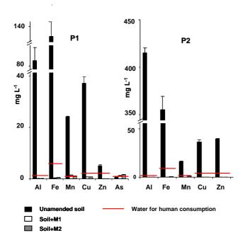
Figure 1 – Metal and As concentration in the leachates from unamended or amended soils (P1 and P2).
