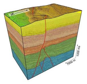
Figure 2 – Surface and subsurface expression of faulting. Blue = Jurassic, Green = Cretaceous, Orange= Eocene, Light orange = Oligocene and Yellow = Miocene.
