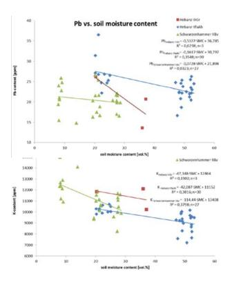
Figure 2 – Moisture dependent XRF-signals exemplified for lead (Pb) (top) and potassium (K) (bottom) of three riparian soil horizons. "SMC" means soil moisture, "R<sup>2</sup>" is measure of determination, and "n" is sample number.
