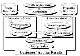
Figure 1 – Overview of the Geological Modeling Process.
