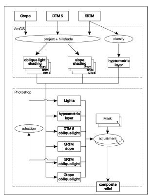
Fig. 3 – Workflow for creating and editing a composite shaded relief
