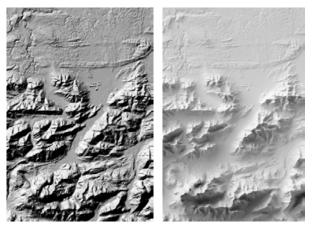
Fig. 5 – left: shaded relief based on SRTM from ArcGIS, right: shaded relief from Blender
