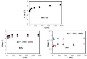
Figure 2 – Kinetic curves for pesticide adsorption on soils
