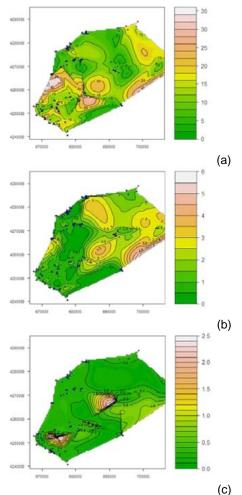
Figure 3 – The spatial prediction maps for the aggregate stability percentage (a); the organic matter percentage (b) and the electrical conductivity values(c).
