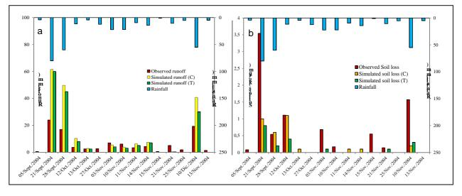
Figure 2 – Comparison of observed and predicted surface runoff (a) and soil loss (b) volumes in the experimental plots (T = treated; C = control).
