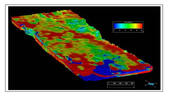
Figure 1: Based on the modeled geological strata so called SGrids can be generated in order to enable voxel-based parametrisation as well as interpolation of attributes throughout the SGrid. Displayed here is the appearance of grain sizes from clay (=red = cohesive layer) to gravel (= blue = non-cohesive layer). Altogether the presented SGrid consists of about 15,000,000 voxels. The area covers about 1,250 km<sup>2</sup> and reaches from Frankfurt in the North to Mannheim in the South.
