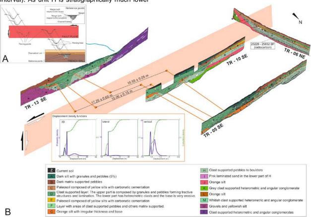
Figure 2. A: Diagram showing the methodology used to calculate buried paleochannel tendency in order to obtain piercing points in the fault plane. B: Three-dimensional model of the El Saltador trenches. Piercing lines, 3D offset measurements and 14C dating are shown.
