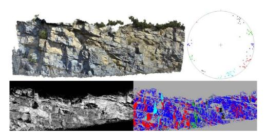
Figure 1 – Upper left: Outcrop orthoimage (length: 27 m Height: 7 m) SfM orthorectification. Upper right: Corresponding stereoplots of the five main fracture sets. Lower left: Laser scanner section with TLS Intensity. Lower right: Point Cloud image after identify and classify surfaces by fracture set orientation SEFL software. Example Middle Eocene Añisclo anticline (Southern Pyrenees).
