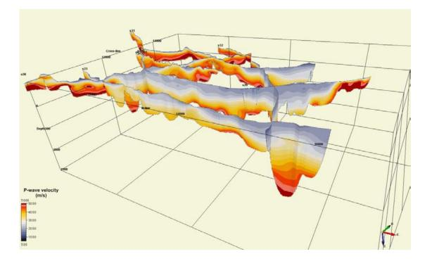
Figure 2 – P-wave velocity models resulting from applying seismic refraction tomography technique.
