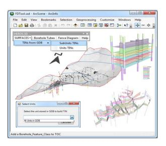
Figure 1. Sketch shows the toolbar implemented in ArcScene (ArcGIS;ESRI) and its main components. Note that some examples of 3D geological surfaces, boreholes and fence diagrams are also shown in the figure.
