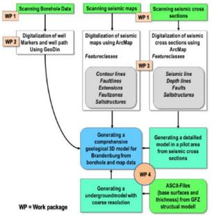
Figure 1 – Workflow for digitization and modelling.
