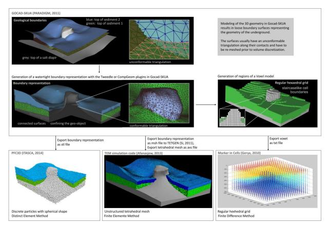
Figure 1 – Preparation of one 3D model produced in Gocad-SKUA for the numerical simulation with 3 different methods. A watertight boundar representation is needed for all simulation methods.
