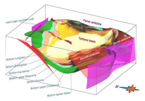
Figure 1 – Geological model of Carrascal-Ferrer Aquifer.
