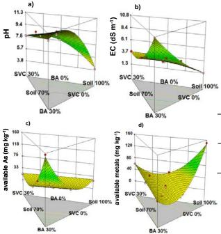
Figure 1 – Surface response plots showing the effect of compost (SVC) and bottom ash (BA) on soil properties: a) pH; b) electrical conductivity; c) As availability and d) metals (AI+Fe+Mn+Cu+Pb+Zn) availability.
