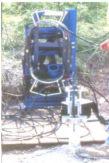
The inclinometric probe at the top of one borehole
