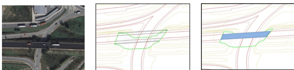
Figure 2 Bridges data capture in the current (left) and in the new (right) models
