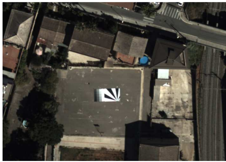
Figure 14. Siemens star quarter used for the resolution study
