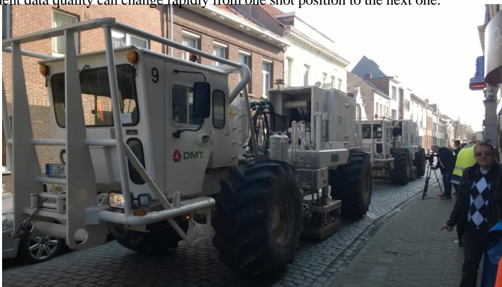
Figure 1 Acquisition of seismic data in an urban environment. Vibroseis trucks are generating seismic signals usually for reflection seismic data processing and interpretation, only.
