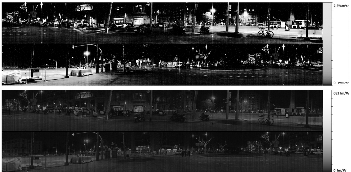
Fig. 6. Top: Integrated radiance ( \text{W m}^{-2} \text{sr}^{-1} ), and bottom: photopic luminous efficacy of radiation (LER) for the nightscape shown in Fig. 5.
